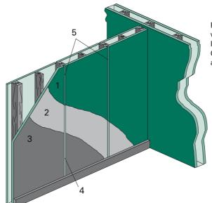
From esthetic point of view CETRIS® boards with chamfered edges can be used. If the customer wishes a surface treatment of CETRIS® boards for to achieve invisible joints, a full area surface filling is necessary.
